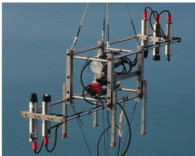
Figure 3. The instrument package used to measure the irradiance quartet and upwelling radiance. As shown, the five radiometric sensors are aligned to the same depth level.
