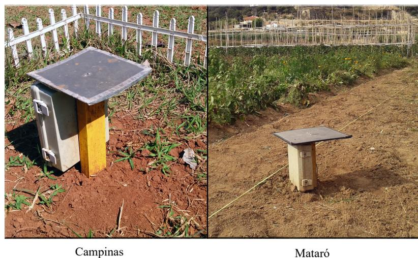
Figure 5. Photographs of the soil temperature profile measurement systems installed in Campinas and Mataró.
