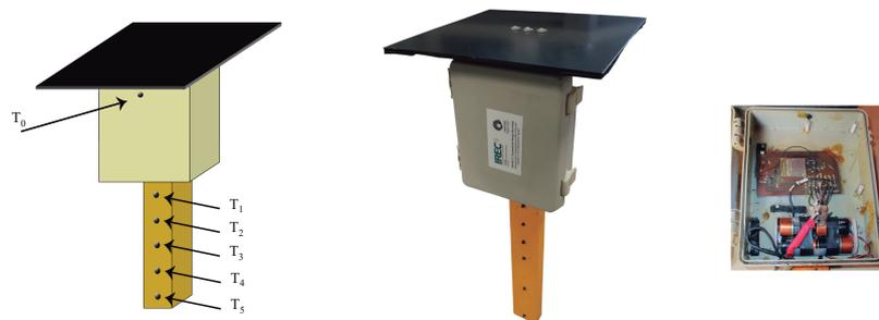
**Figure 2.** Sketch and photograph of the flat panel with temperature sensor and data-logger.
