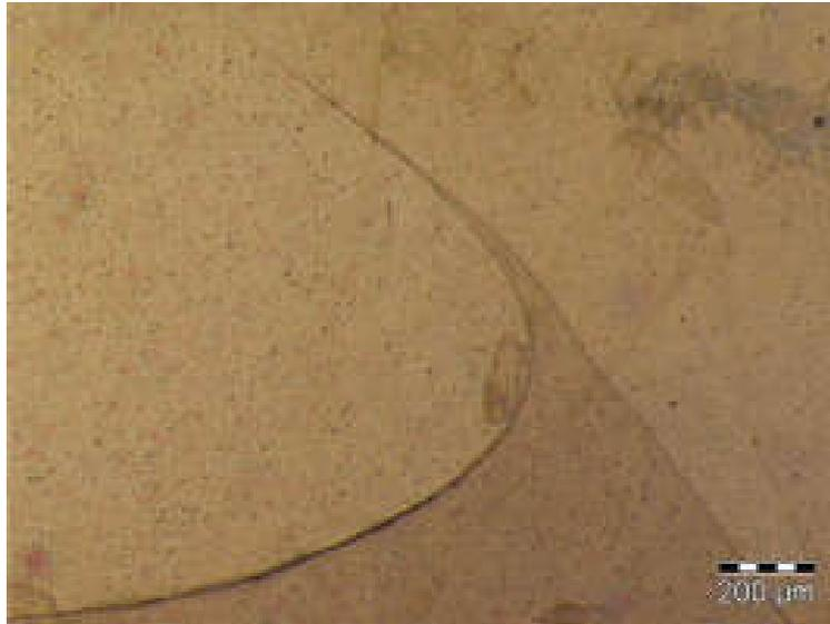
**Figure 11.** Hook defect of the dissimilar joint (AA5754-AA6082) [82].
