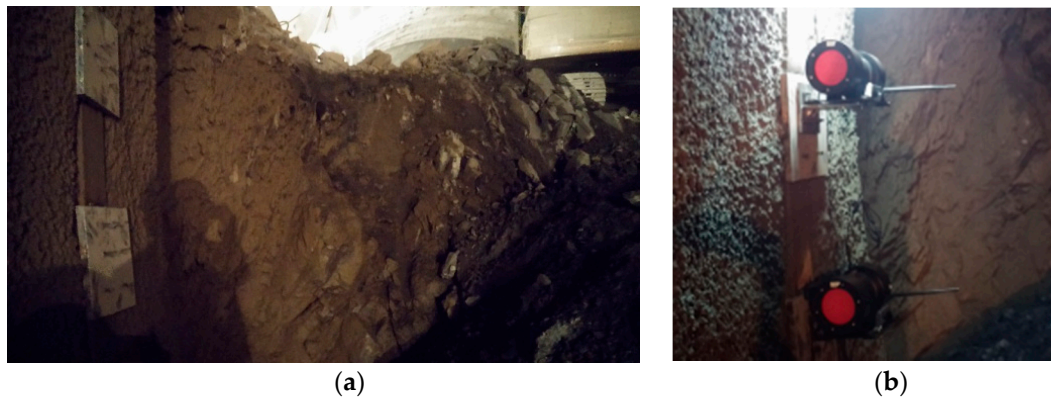
Figure 26. (a) Measured points; (b) image acquisition module mounted on measured points.
