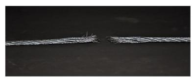
$(\boldsymbol{a})$  The broken rope defect of the steel cord conveyor belt
