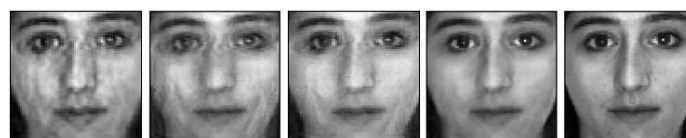
Figure 4. Enlarged restored images. From left to right, it is the restored images of DnCNN, ResNet, ResNet with dilated convolution and FbResNet, and the last is the clean image.
