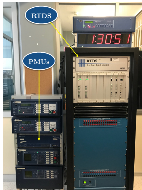
Figure 3. Hardware-in-the-loop implementation in RTDS.
