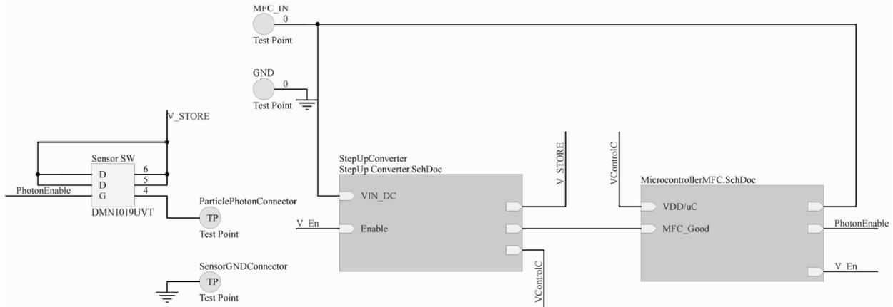
**Figure 1.** Power management system circuit for multiple microbial fuel cells.
