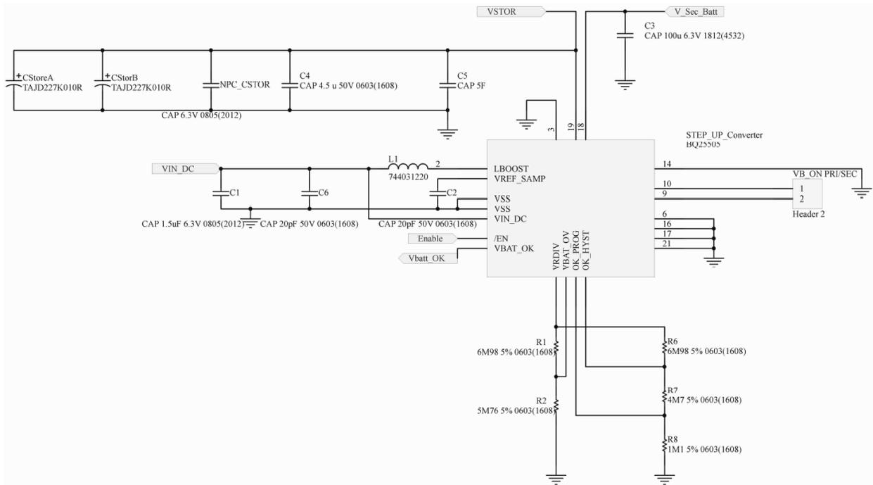
**Figure 3.** Step-Up Converter block schematic.
