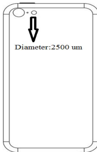
Figure 3. The BM photoresist build-up dimension (nominal-the-best; diameter: 2500  $\mu\text{m}$ ).
