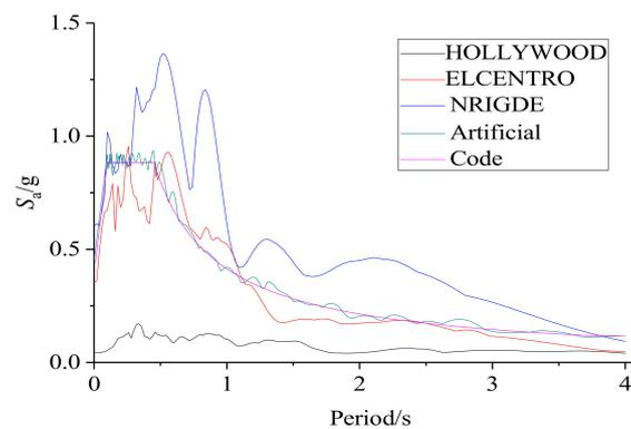
**Figure 13.** Response spectra of seismic waves.
