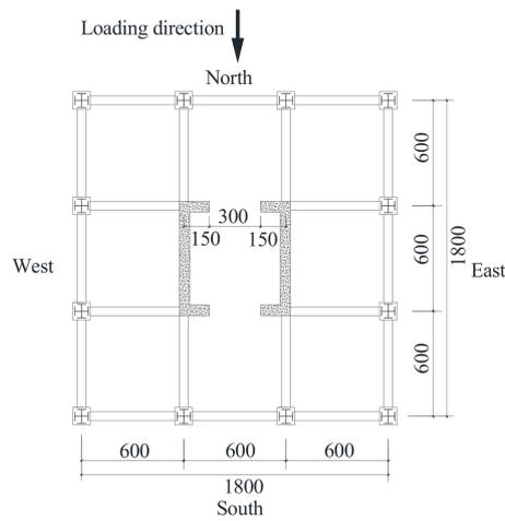
Figure 1. Plan arrangement (units: mm).
