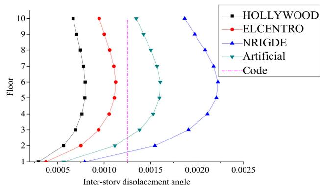
Figure 18. Inter-story displacement angle in case 1.
