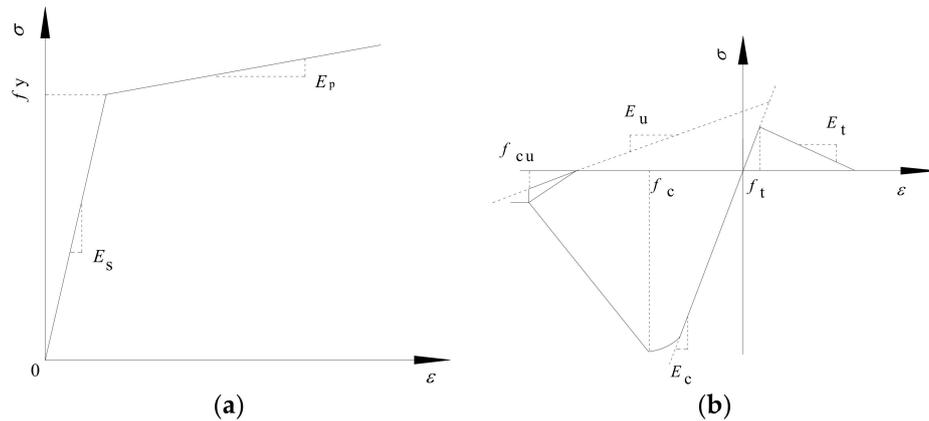
**Figure 7.** Constitutive model of materials: (a) constitutive model of steel and (b) constitutive model of concrete.
