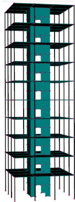
Figure 9. The finite element (FE) model.
