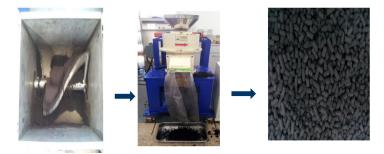
**Figure 1.** Processing diagram of the biochar pellet with different combinations of biochar and pig manure compost described by Shin et al. (2018) [26].
