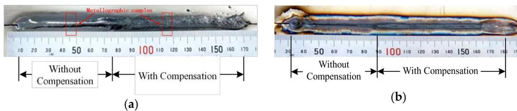
Figure 5. Weld bead shape of sample 1#: (a) Front view; (b) back view.
