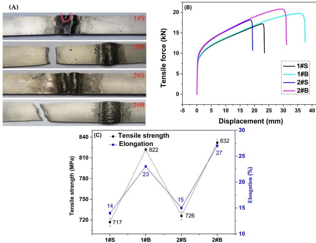
**Figure 11.** Tensile properties of welded joints: (A) Tensile samples; (B) tensile curves; (C) result of tensile tests.
