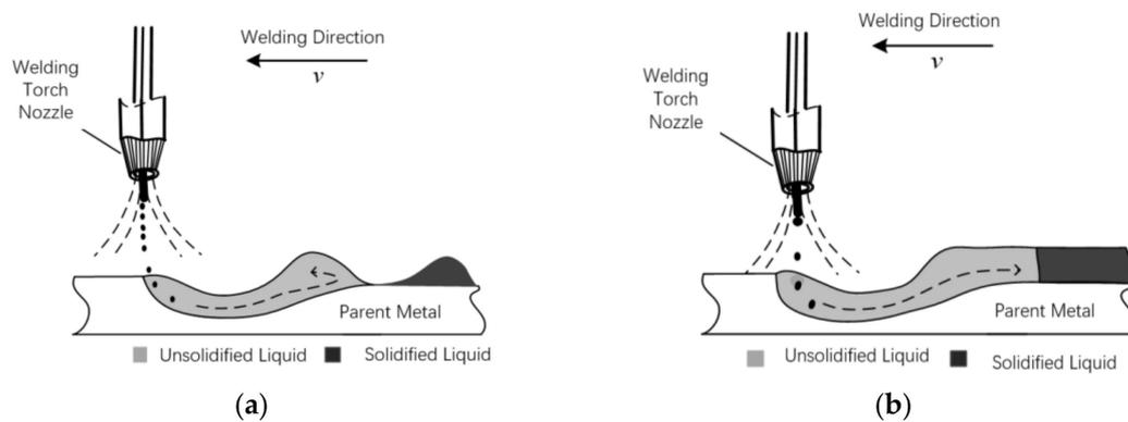
**Figure 1.** Schematic of the relative speeds of molten steel flows and parent material: (a) Low relative speed (high-speed welding); (b) high relative speed (normal welding).
