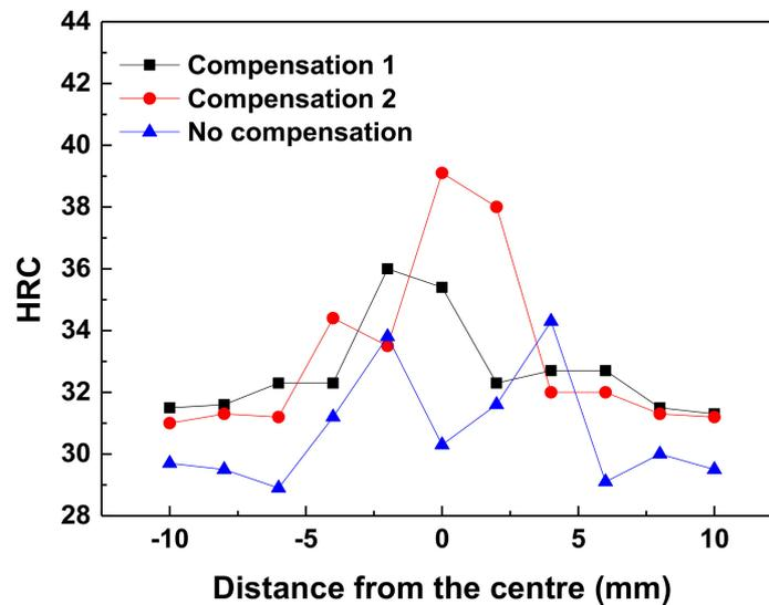
Figure 9. Comparison of hardness curves of welds formed with and without compensatory gas jets.
