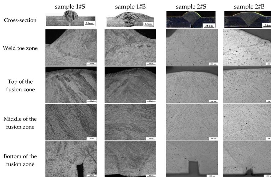
**Figure 7.** Microstructures of butt welds formed at high-speed welding.
