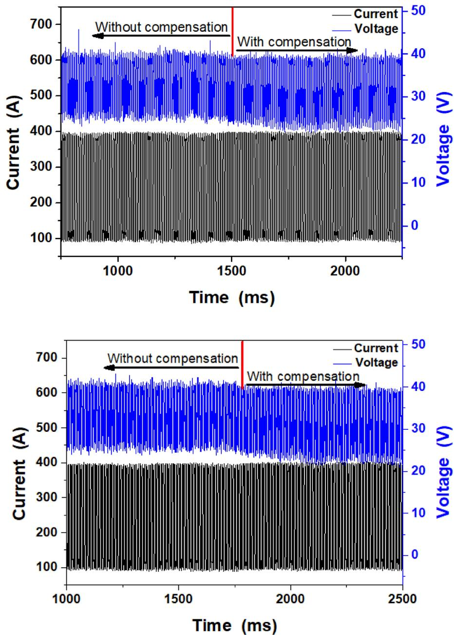
Figure 4. Current and voltage waveforms during the butt welding of 304 stainless steel: (a) Sample 1#; (b) sample 2#.
