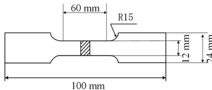
Figure 10. Dimensions of tensile strength test specimens.
