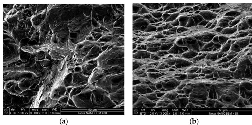
**Figure 12.** Photographs of fractured tensile samples: (a) Weld joint, (b) base material.
