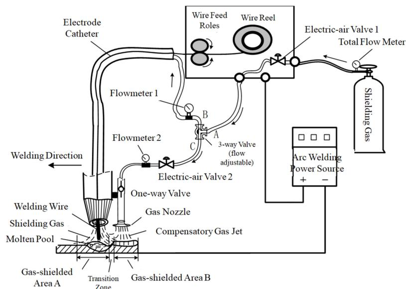
Figure 2. Schematic of the molten pool blown with compensatory gas jet during welding.
