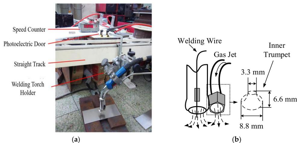
Figure 3. Self-made compensatory gas jet test platform: (a) Diagram of the compensatory gas jet system; (b) diagram of compensatory gas jet nozzle structure.
