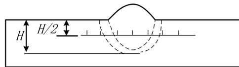
Figure 8. Weld hardness test point.
