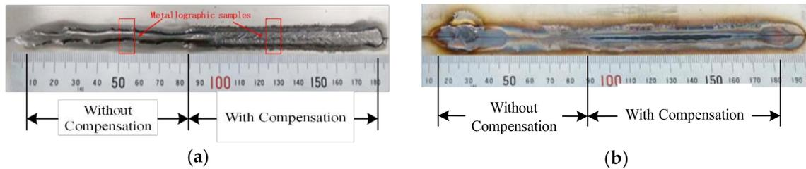
Figure 6. Weld bead shape of sample 2#: (a) Front view; (b) back view.
