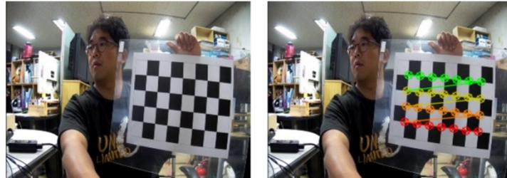
**Figure 4.** Feature point extraction using a chess board.
