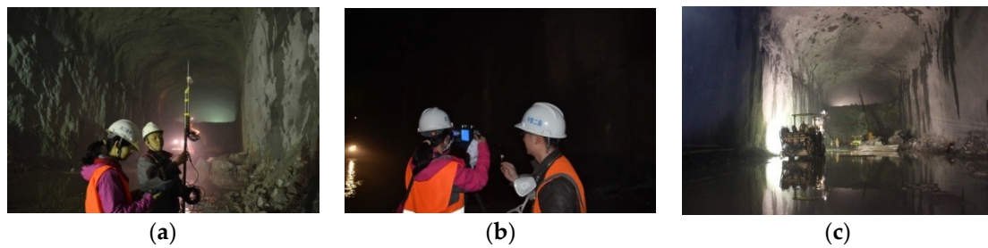
Figure 4. Field test of ventilation environment in the caverns: (a) Test of air velocity; (b) Test of dust; (c) Air quality after ventilation.
