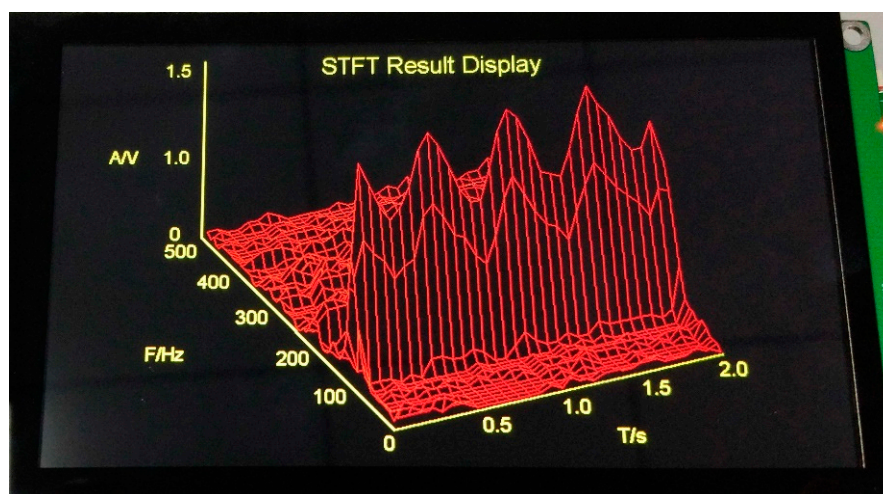
Figure 9. Spectrogram of fault vibration signal, generated by an embedded device.
