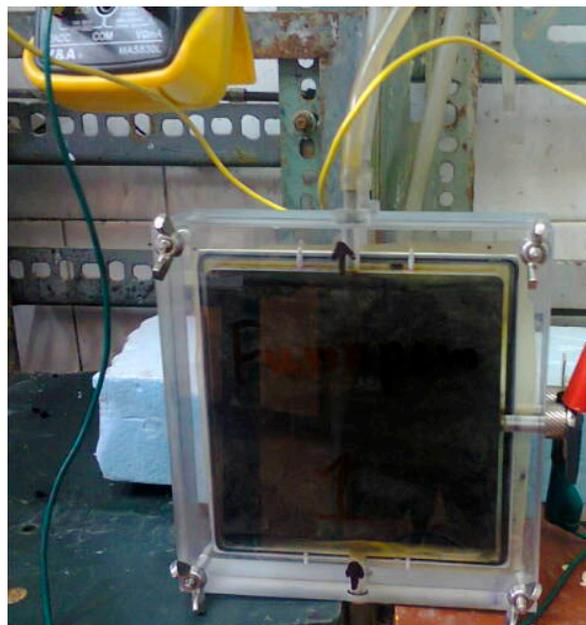
Figure 6. Experimental set-up of a single rectangular fuel cell with 100 sq/cm electrode and membrane area.
