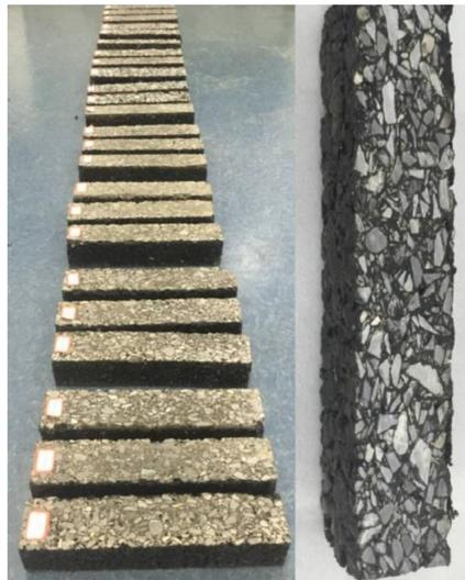
**Figure 3.** Beam-shaped specimens prepared for the fatigue test.
