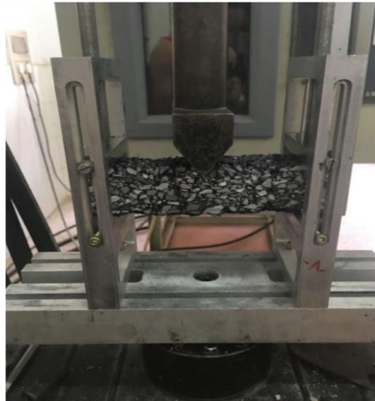
Figure 4. Fatigue test.
