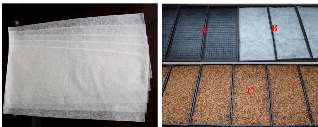
Figure 1. (left) The ramie fiber/starch nonwoven film; and (right) Its application. A: Empty plate for raising rice seedlings for machine-transplanting, B: The film is padded on the bottom surface of the plate, C: The film is covered with cultivated soil and rice seeds are sown on it.
