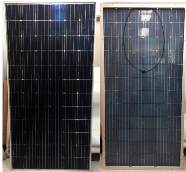
Figure 20. The 72-cell Si bifacial photovoltaic (PV) module used in application test.
