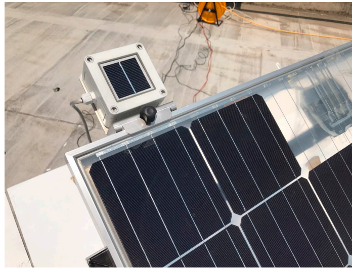
Figure 17. Pyranometer installed on the back of the modules.
