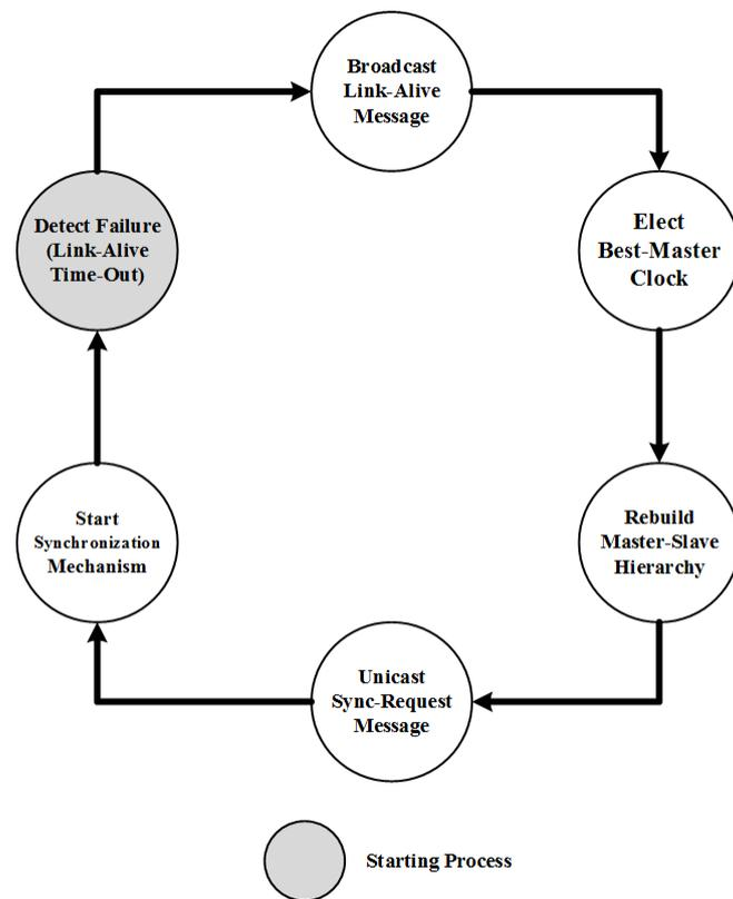
Figure 4. The TFR process. TFR: timing fault recovery.
