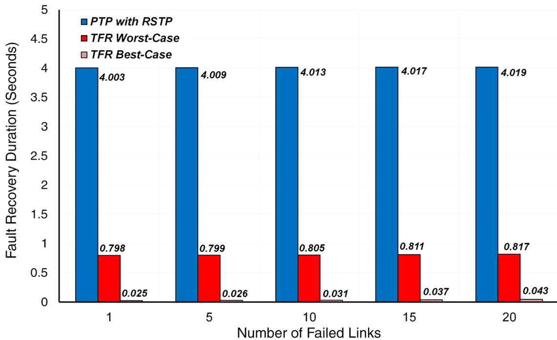
**Figure 8.** A simulation comparison of fault recovery durations in the TFR and PTP under RSTP approaches. TFR: Timing Fault Recovery; RSTP: Rapid Spanning Tree Protocol.
