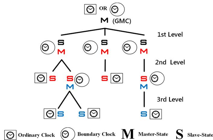
**Figure 1.** Example of the PTP master–slave synchronization hierarchy. PTP: Precision Time Protocol; GMC: grandmaster clock.
