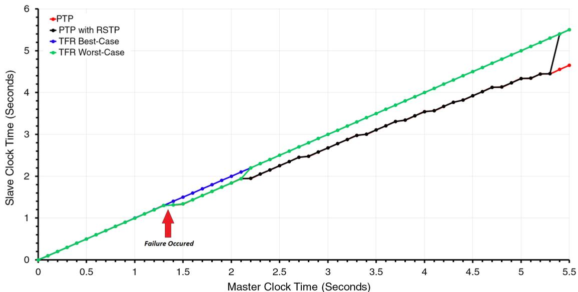
**Figure 9.** Slave clock timing values with TFR and PTP with RSTP with respect to MC timing. MC: Master Clock.
