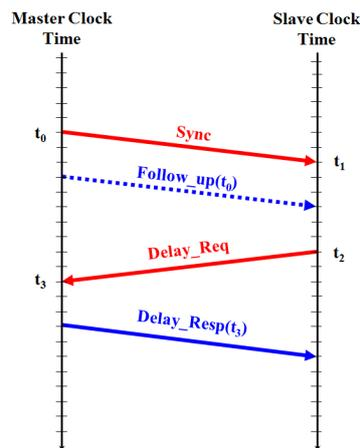
**Figure 3.** Delay request–response mechanism of the PTP timing exchange protocol.
