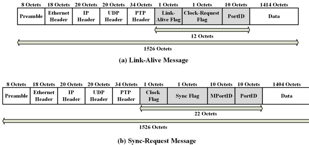
**Figure 5.** The structures of the Link-Alive and Sync-Request messages. IP: Internet Protocol; UDP: User Datagram Protocol.
