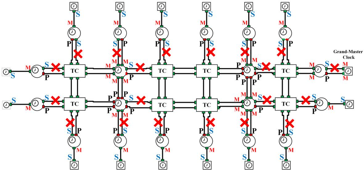
Figure 7. A sample PTP network with possible link failures.
