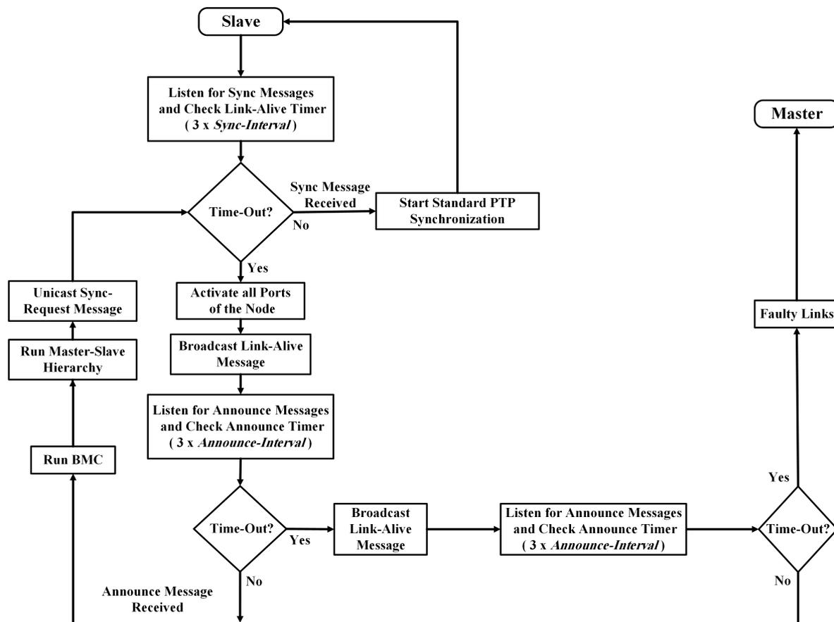
Figure 6. The TFR state machine. BMC: best master clock.
