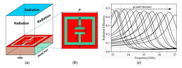
**Figure 4.** The complementary electric-field-coupled (CELC) element with a unit cell size of 2 mm: (a) full-wave simulation model; (b) its top view; (c) the variation in radiation efficiency when *l* and *g* change.
