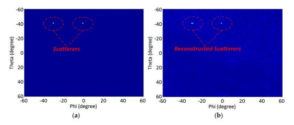
**Figure 9.** Target scenes: (**a**) true target scene consisting of two point scatterers; (**b**) the same scene reconstructed by the fabricated MAA.
