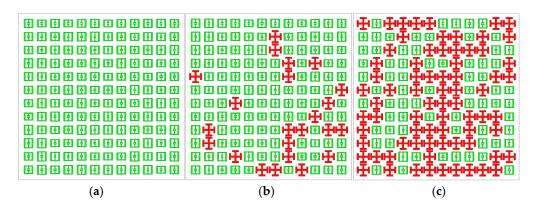
**Figure 6.** The schematic of simulated metamaterial aperture antenna (MAA) with different ratios of CJC elements: (**a**) 0%; (**b**) 20%; (**c**) 50%.
