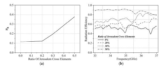
**Figure 7.** (a) Calculated average mutual coherence  $\mu_g$  and (b) the radiation efficiency of different MAAs with different filling ratios of CJC elements.
