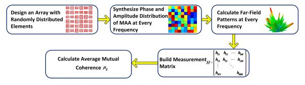
**Figure 2.** Flow chart of the  $\mu_g$  analysis procedure.
