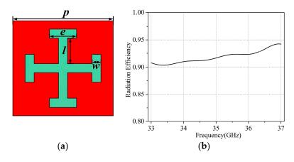
**Figure 5.** (a) Top view of complementary Jerusalem cross (CJC) element with a unit cell size of 2 mm and (b) a radiation efficiency of the element.
