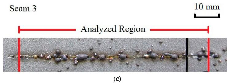
Figure 3. Welded seams of different welding speeds: (a) 3 m/min; (b) 4.5 m/min; (c) 6 m/min.
