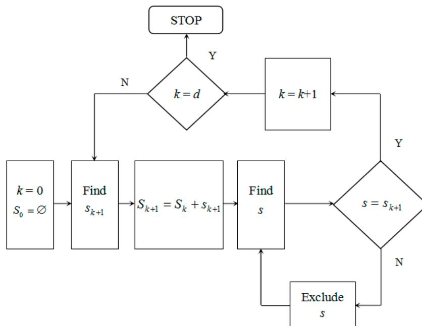
Figure 1. The flow chart of SFFS algorithm.
