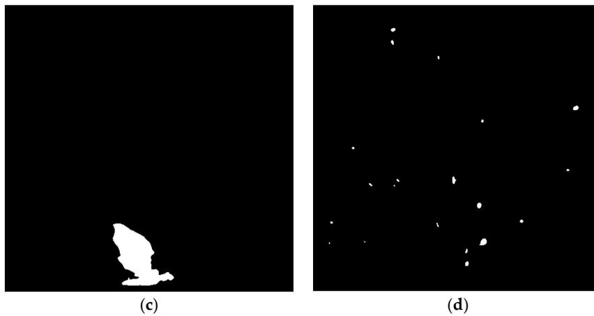
**Figure 2.** Schematic diagrams of image processing: (a) original image; (b) grayscale image; (c) binary image of plume; (d) binary image of spatters.
