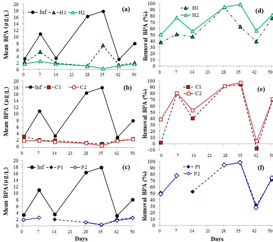
**Figure 2.** Longitudinal BPA concentrations in CWs of (a) *Heliconia* (H); (b) unplanted control (C), and (c) *Phragmites* (P), for influent (Inf), two-thirds internal (1), and effluent (2) sample points. Removal efficiency of BPA in (d) *Heliconia*; (e) unplanted control; and (f) *Phragmites*.
