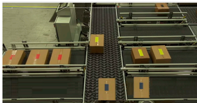
Figure 2. The example of an AMHS (Automated Material Handling System) with ARB (Activated Roller Belt) conveyor.
