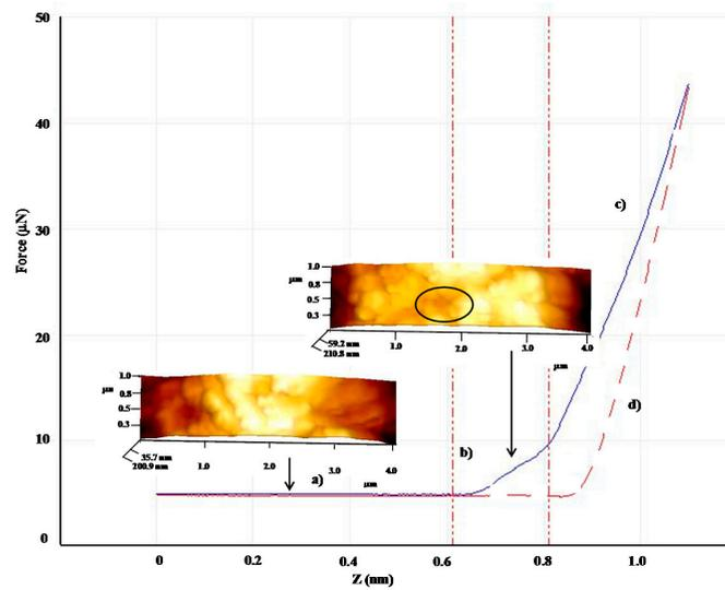
**Figure 6.** Mechanical testing of the elastic-plastic region by AFM of the MPCM composed by PS:tetracosane (1:3) microcapsule at 60 °C: (a) no contact, continuous line; (b) plastic penetration; (c) deformation of the sample; and (d) retraction of the AFM probe, discontinuous line.
