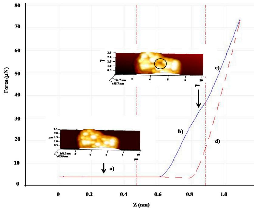
**Figure 3.** Mechanical testing of the elastic-plastic region by AFM of the MPCM composed by PMMA:tetracosane (1:3) microcapsule at 23 °C: (a) image of the sample before applying forces, no contact; (b) change in the slope, defined as the maximum force that can be applied to the sample ; (c) deformation of the sample; (d) retraction of the AFM probe until there is no contact between the tip and the sample.
