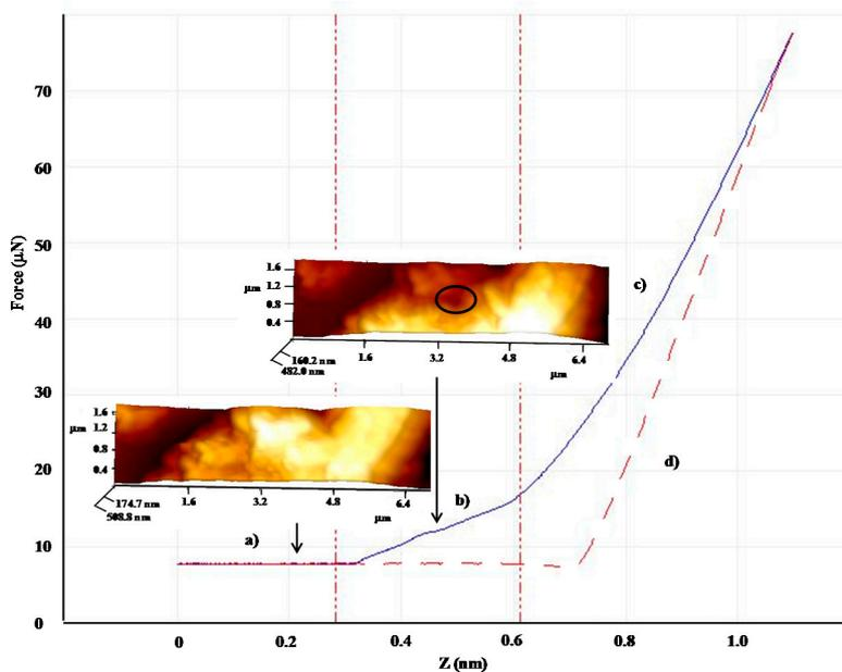
**Figure 5.** Mechanical testing of the elastic-plastic region by AFM of the MPCM composed by PS:tetracosane (1:3) microcapsule at 23 °C: (a) no contact, continuous line; (b) plastic penetration; (c) deformation of the sample; and (d) retraction of the AFM probe, discontinuous line.
