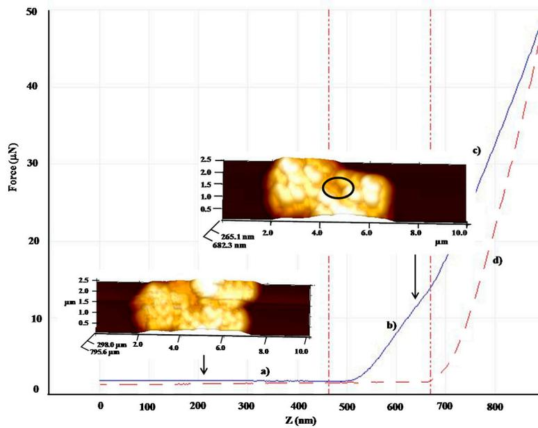
**Figure 4.** Mechanical testing of the elastic-plastic region by AFM of the MPCM composed by PMMA:tetracosane (1:3) microcapsule at 60 °C: (a) no contact, blue continuous line; (b) plastic penetration; (c) deformation of the sample; and (d) retraction of the AFM probe, red discontinuous line.
