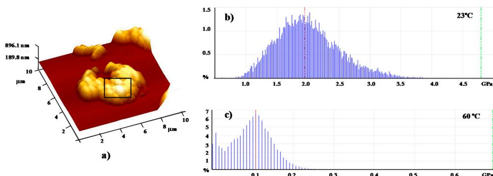
**Figure 1.** Results for PMMA:tetracosane (1:3): (a) 3D image tested; (b) Effective Young's modulus results at 23 °C; (c) Effective Young's modulus results at 60 °C.
