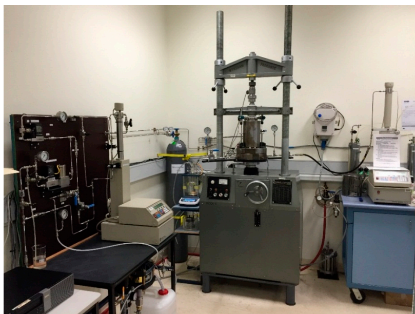
Figure 2. High-pressure triaxial setup used to conduct fracturing and permeability tests.
