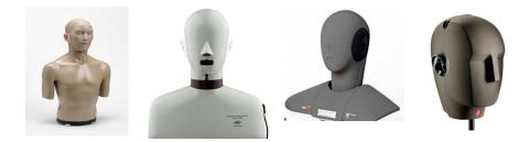
**Figure 4.** Dummy heads (from left to right): KEMAR, Brüel & Kjær 4128 HATS, Head Acoustics HMS III, and Neumann KU-100. Note that Neumann KU-100 dummy head is torso-free.
