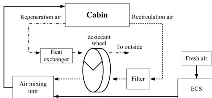
**Figure 1.** Desiccant wheel-based air purification system diagram.
