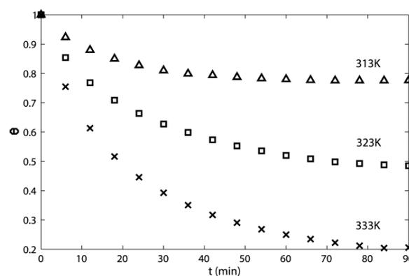
**Figure 6.** Toluene thermal desorption curves of silica gel.
