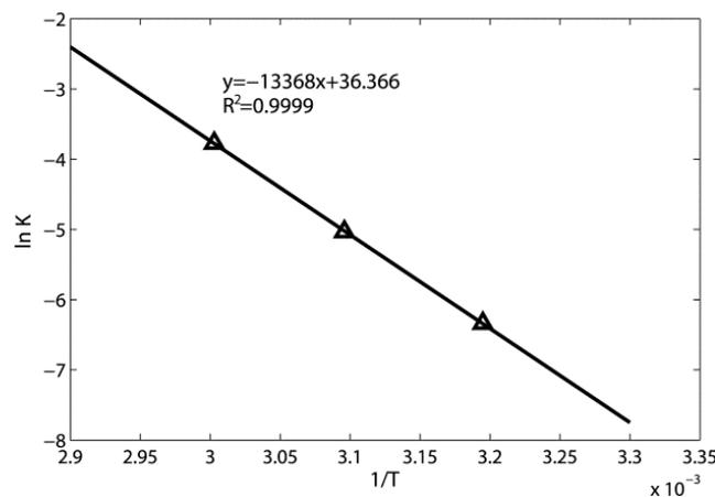
**Figure 8.** The Van't Hoff plot for equilibrium constant of silica gel thermal desorption.
