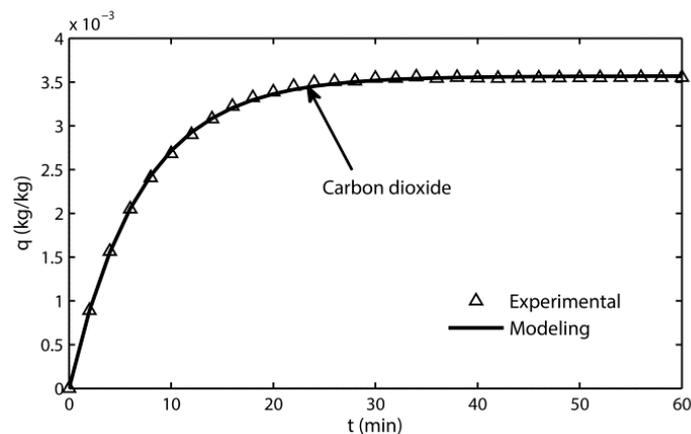
Figure 3. Experimental and modeling adsorption curves for carbon dioxide.
