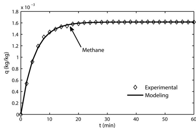
Figure 4. Experimental and modeling adsorption curves for methane.
