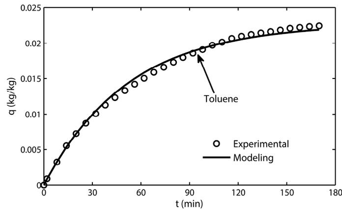
Figure 5. Experimental and modeling adsorption curves for toluene.
