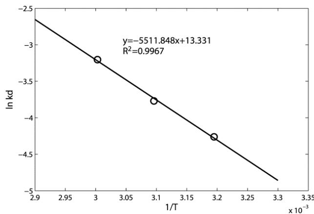
**Figure 7.** The Arrhenius plot for reaction constants of silica gel thermal desorption.
