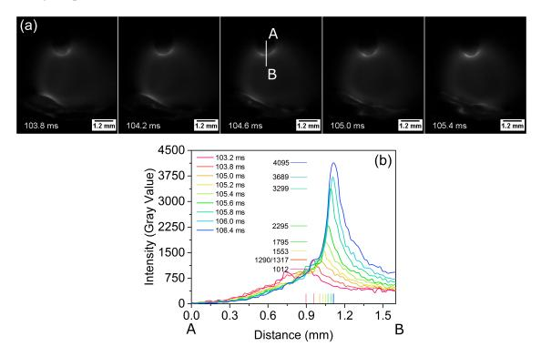
**Figure 2.** Pixel intensity at wire tip for a current of 55 A, observed with an aperture of f/22 using at narrow band pass filter of  $515 \pm 10$  nm wavelength and exposure time of  $80 \,\mu$ s: (**a**) frames of the high speed image, (**b**) pixel intensity plotted.
