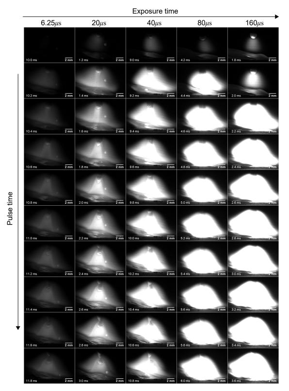
**Figure 3.** Arc appearance for aperture of f/22 using at narrow band pass filter of 900  $\pm$  10 nm wavelength for different camera sensor exposure times.
