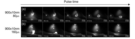
**Figure 5.** Bandpass filters and exposure times that can be used for (**a**) droplet temperature measurement and (**b**) weld pool behavior (current 50 A) captured using different bandpass filters and exposure times.
