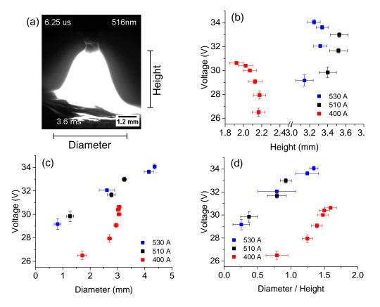
**Figure 8.** (a) schematic geometric features measured; variation of welding voltage with metal vapor column (b) height, (c) diameter at the cathode, and (d) ratio between diameter and height. The high-speed images were taken using the  $515 \pm 10$  nm wavelength filter, exposure time of 6.25 µs, and lens aperture of f/22.
