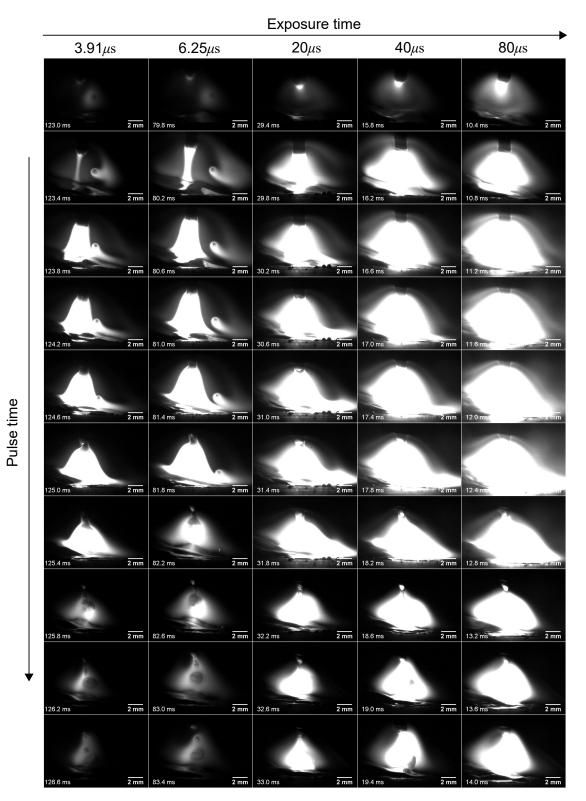
**Figure 1.** Arc appearance for aperture of f/22 using at narrow band pass filter of  $515 \pm 10$  nm wavelength for different camera sensor exposure times.
