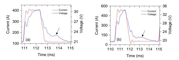
Figure 6. Variation of current and voltage for peak current of (a) 400 A and (b) 530 A.
