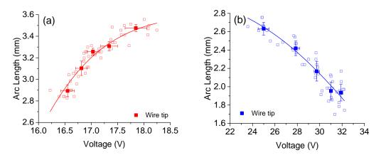
Figure 7. Variation of welding voltage with arc length for current values of (a) 50 A and (b) 380 A.
