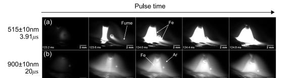
**Figure 4.** Iron (Fe) metal vapour and argon (Ar) dominated regions during pulse peak phase (current of 400 A) captured using different bandpass filters and exposure times: (**a**)  $515 \pm 10$  nm filter and exposure time of  $3.91 \,\mu$ s, (**b**)  $900 \pm 10$  nm filter and exposure time of  $20 \,\mu$ s.
