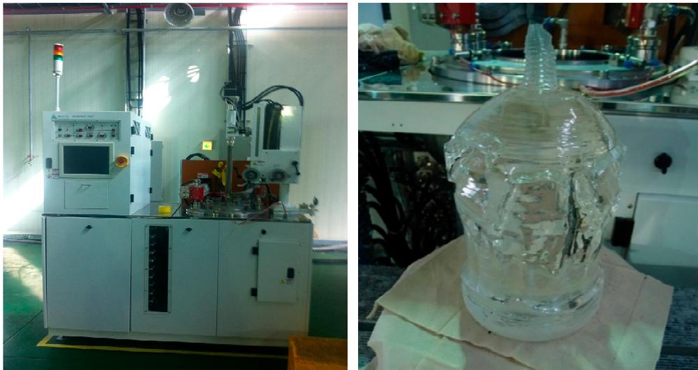
Figure 7. The single crystal growth of sapphire using the Ky method.
