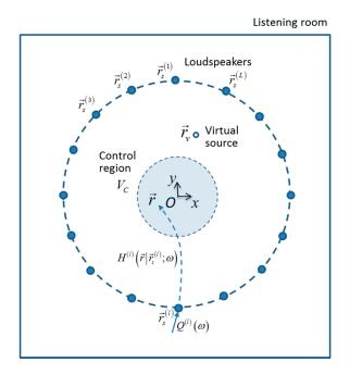
Figure 1. A typical sound field reproduction system in a listening room.
