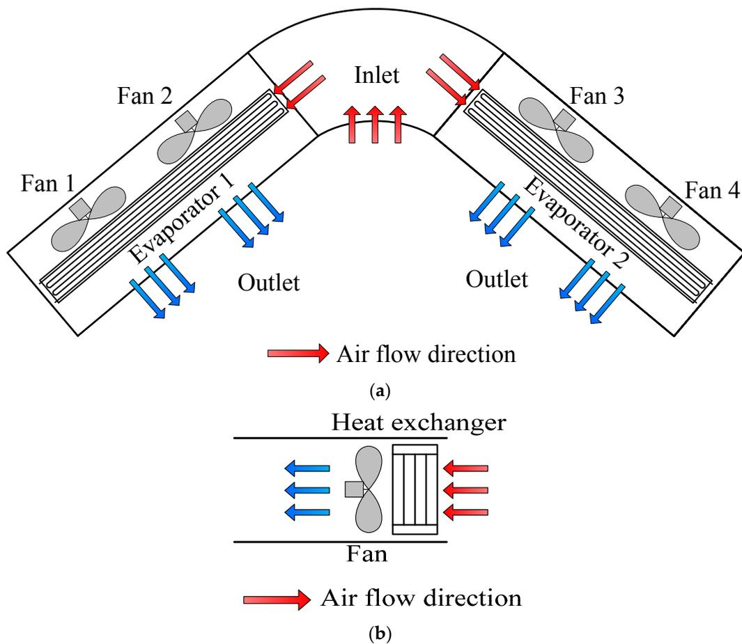
**Figure 2.** Schematic diagrams of the evaporator and condenser parts. (a) One section of the evaporator part; (b) Condenser part.
