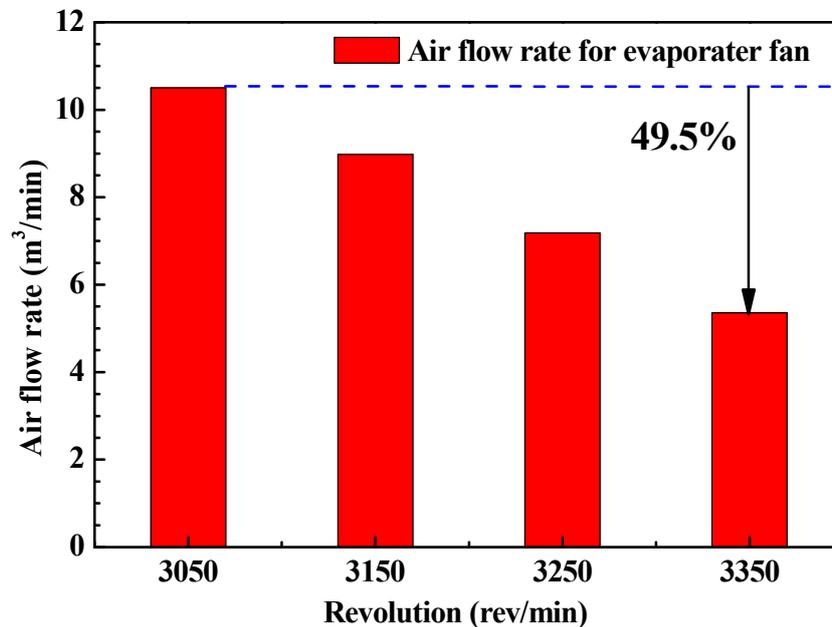
Figure 3. Air flow rate of the evaporator fan with fan rotation speeds.
