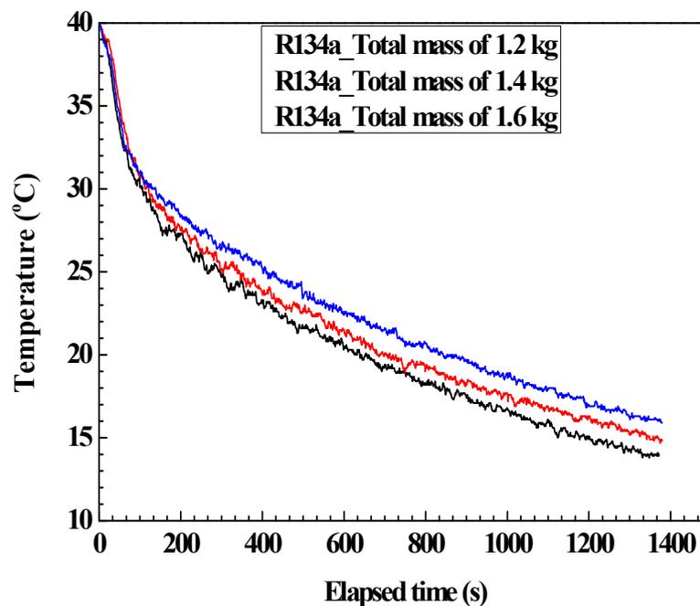
**Figure 4.** Cooling speeds of the two parallel refrigeration cycles with the refrigerant charge amount for a special purpose vehicle.
