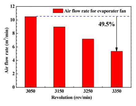
Figure 3. Air flow rate of the evaporator fan with fan rotation speeds.
