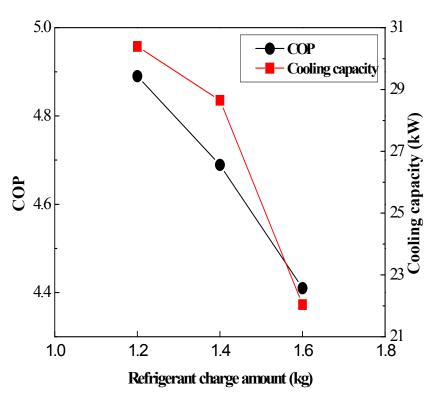
**Figure 5.** Cooling capacity and COP of the two parallel refrigeration cycles with the refrigerant charge amount for a special purpose vehicle.
