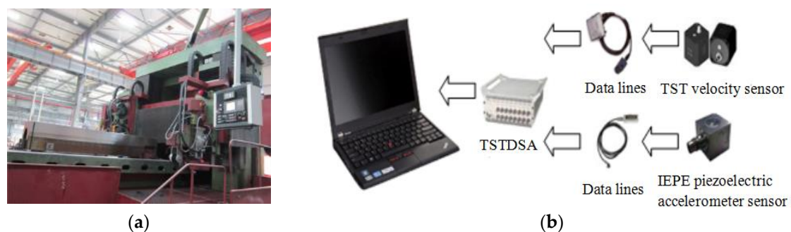
Figure 11. (a) CNC guideway grinder KD4020X16; (b) TST5912 analysis system.
