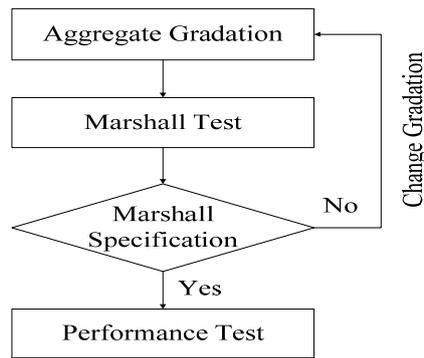
Figure 1. Flow chart of stone matrix asphalt (SMA) mixture design.
