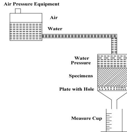
Figure 2. Schematic of the permeability test device.
