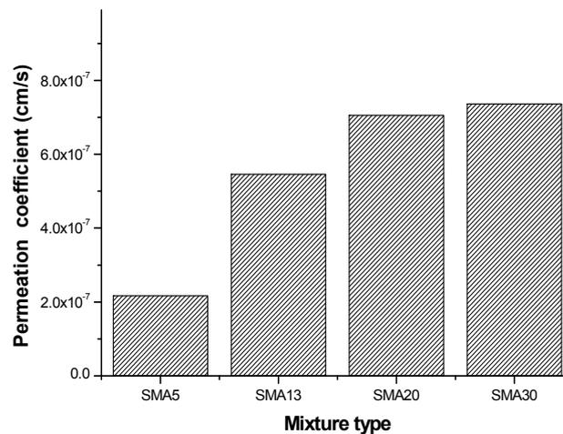
Figure 3. Mixture types and permeability coefficients.
