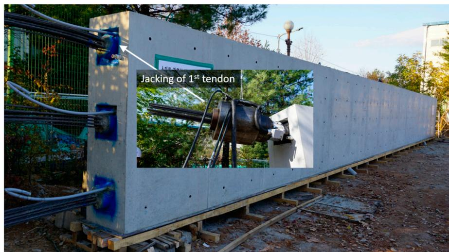
Figure 7. Shape of specimen and jacking process.
