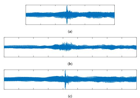
**Figure 7.** An example of the proposed transient preservation method. (**a**) shows the original audio, consisting of a solo violin overlaid with a castanet click. Also shown are the modified samples with TSM factor  $\alpha = 1.5$ , using (**b**) the standard phase vocoder, and (**c**) the proposed method.
