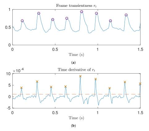
**Figure 6.** Illustration of the proposed transient detection. (**a**) Frame transientness. Locations of the detected transients are marked with purple circles; (**b**) Time derivative of the frame transientness. Detected transient onsets are marked with orange crosses. The red dashed line shows the transient detection threshold.
