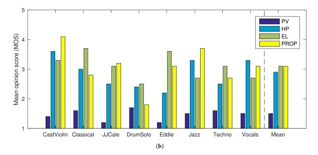
**Figure 8.** Mean opinion scores for eight audio samples using four TSM methods for (**a**) medium ( $\alpha = 1.5$ ), and (**b**) large ( $\alpha = 2.0$ ) TSM factors. The rightmost bars show the average score for all eight samples. PV: phase vocoder; HP: harmonic–percussive separation [28]; EL: élastique [36]; PROP: proposed method.
