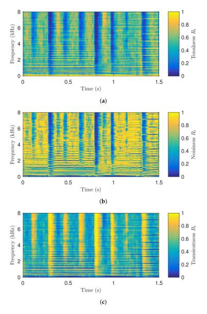
**Figure 4.** (**a**) Tonalness, (**b**) noisiness, and (**c**) transientness values for the short-time Fourier transform (STFT) bins of the example audio signal. Cf. Figure 1.
