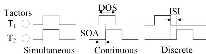
**Figure 4.** Schematic diagram of tactile apparent motion.
