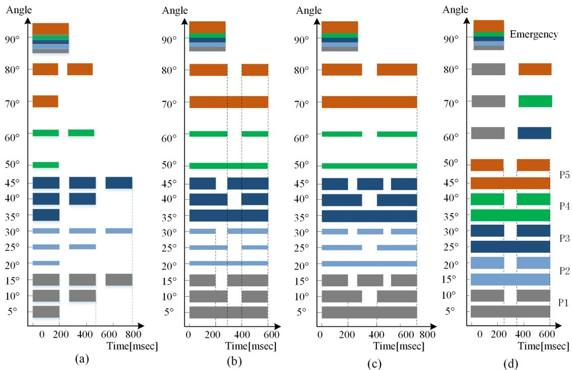
**Figure 8.** Schematic diagram of coding methods with combination of three parameters: (a) location, rhythm of times and intensity (LRI1); (b) location, rhythm of duration and intensity (LRI2); (c) location, rhythm of times and intensity (LRI3); (d) location, rhythm and mode (LRM). For the convenience of labelling angel intervals, five degrees in vertical coordinate indicates the interval [5, 10) in Table 3, 10 indicates [10, 15) and so forth.
