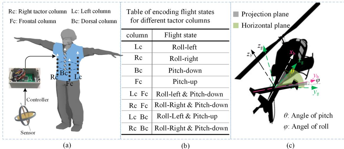
**Figure 3.** Overview of vibrotactile system for cueing flight attitude. (a) System block diagram of vibrotactile TSAS and Tactor arrangement around the torso of pilot. The controller receive flight attitude information from the geomagnetic sensor and activate vibrotactile vest to vibrate in the pattern corresponding to the attitude; (b) Schematic diagram of encoding flight states for different tactor columns; (c) Definition of Flight attitude information of aircraft.
