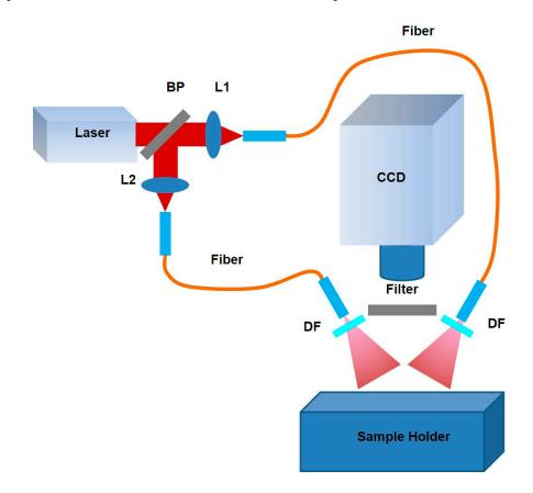
Figure 3. Near-Infrared planar fluorescence imaging system. BP, beam splitter; L1, L2, lens; DF, diffuser.
