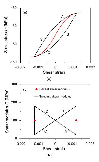
Figure 2. Evolution of the shear modulus along the  $A \to B \to C \to D$  loading path for the given shear strain amplitudes of  $\Delta \gamma = 1.2 \times 10^{-3}$ . (a) Hysteresis loop and (b) Shear modulus. The tangent shear modulus is calculated from Equation (2). Circles indicate the secant shear modulus. Note that  $G_{sec}(\Delta \gamma)$  is equal to the average of the tangent moduli at  $\pm \gamma$ .
