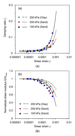
**Figure 3.** Strain-dependent behavior of sand and clay under different confinement stress levels: (a) Damping ratio and (b) Secant shear modulus. The symbols are experimental data and the lines are defined by Equations (8) and (4). The symbols are experimental data [31].
