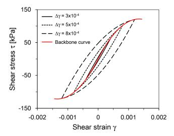
**Figure 1.** Nonlinear stress-strain behavior of soil subjected to three different shear strain amplitudes. The hysteretic loops and backbone curve are obtained using Equations (1) and (3). The model parameters are  $G_{\text{max}} = 180 \text{ MPa}$ ,  $\alpha = 370$ , and n = 2.
