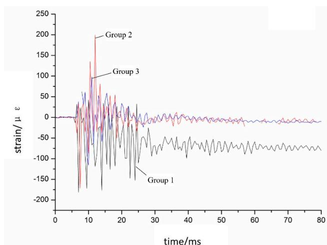
**Figure 28.** Data from JFBGS-200 concrete surface strain gauges (position No. 7).
