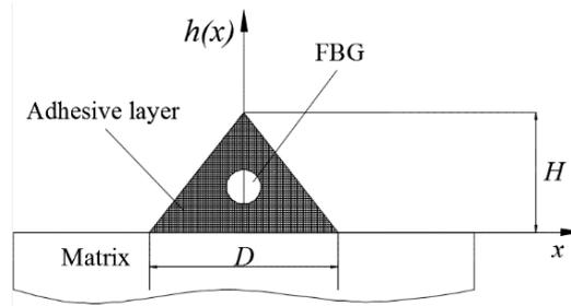
Figure 5. The model of the surface-bonded fiber.
