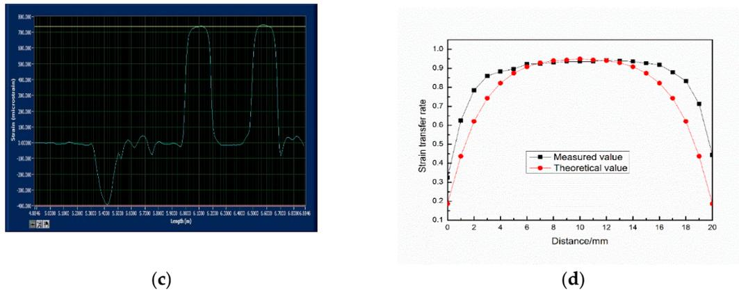
**Figure 3.** The strain transfer experiment of the soft layer encapsulated fiber with the distributed sensing interrogator ODISI OBR 4600. (a) The LUNA OBR 4600 distributed sensing system; (b) Fiber bonded to the cantilever beam; (c) Strain measured by OBR 4600 along the fiber; and (d) Strain transfer measured in contrast to strain transfer ratio calculated based on the theoretical strain transfer model.
