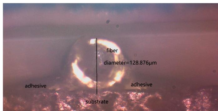
**Figure 4.** The cross section of the surface bonded bare Polyimide FBG.
