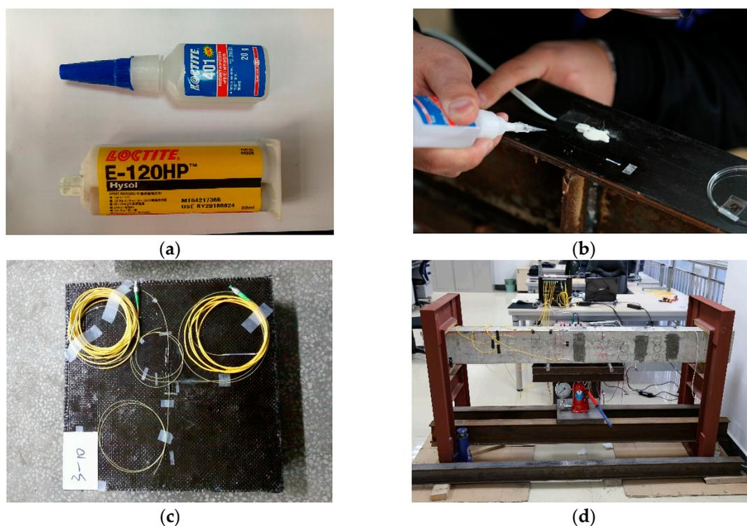
**Figure 13.** Bonding method. (a) Loctite 401 and E-120HP; (b) Bare polyimide FBG was bonded to the CFRP (Carbon Fiber Reinforced Polymer) plate by Loctite 401; (c) Bare polyimide FBGs were bonded to the CFRP textile by Loctite 401 first and then covered by E-120HP; (d) Bare polyimide FBGs were bonded to the concrete specimen by Loctite 401 first and were then covered by E-120HP.
