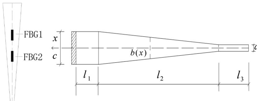
Figure 20. Cantilever beam and bonding diagram.
