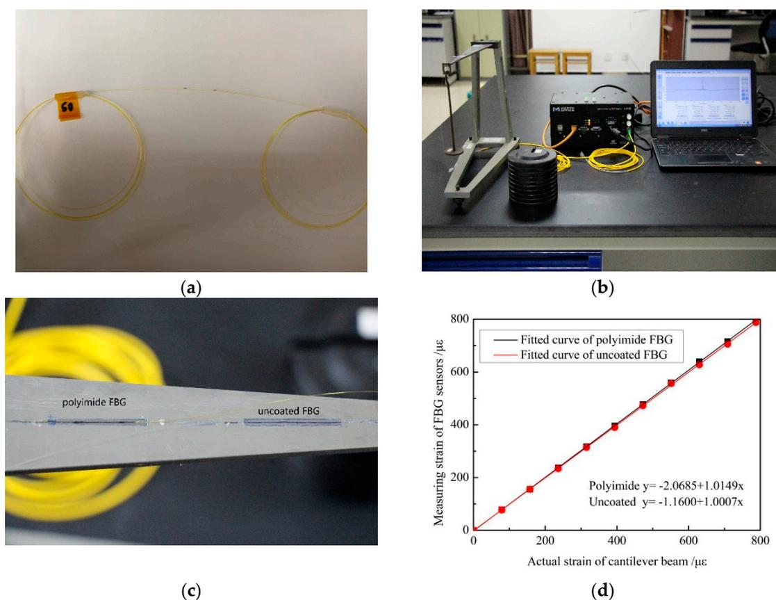
**Figure 1.** Samples of polyimide fiber Bragg gratings (FBGs). (a) Bare Polyimide FBG; (b) Strain transfer ratio experiment for polyimide FBG and uncoated FBG; (c) Bonding types for comparison; (d) Results of strain measured by polyimide FBG and uncoated FBG.
