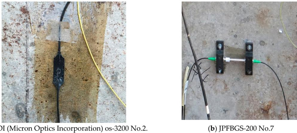
Figure 24. Photos of os-3200 non-metallic and JPFBS-200 optical strain gauges.
