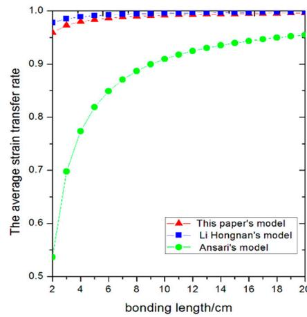
Figure 8. Average strain transfer ratios of different models.
