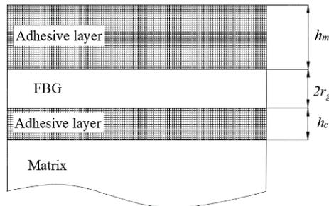
Figure 6. The structure of surface-bonded fiber.
