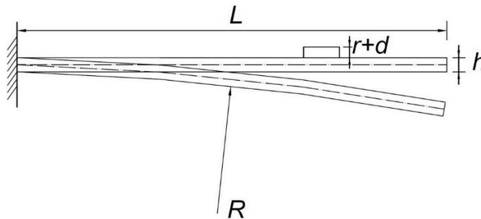
**Figure 15.** Diagram of the FBG pasted on the cantilever beam.
