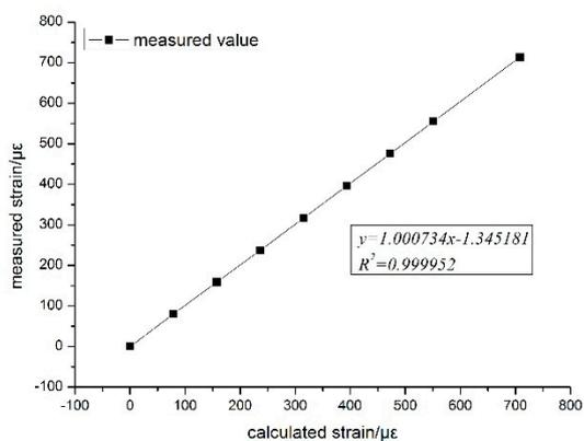
Figure 16. The unrevised average strain transfer rate of the FBG (1570 nm).
