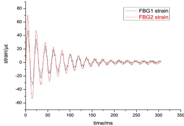
**Figure 21.** Strain of the cantilever beam measured by FBGs.
