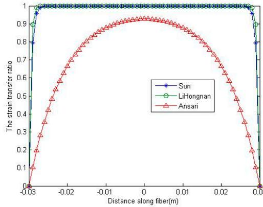
Figure 7. Strain transfer ratio along the gauge length of FBGs of different models.
