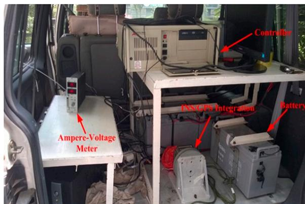
Figure 12. The vehicle loaded navigation equipment.
