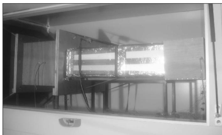
**Figure 2.** Photograph of the storage component installed in the closed-loop air-supply system.
