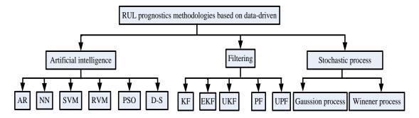
**Figure 1.** The main remaining useful life (RUL) prognostics methodologies of vehicle lithium-ion batteries.
