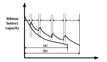
**Figure 2.** Lithium battery capacity changing with discharge process. (**a**) Continuous discharge; (**b**) intermittent discharge.
