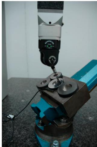
**Figure 3.** Measurements of standard ring in one of the selected positions.
