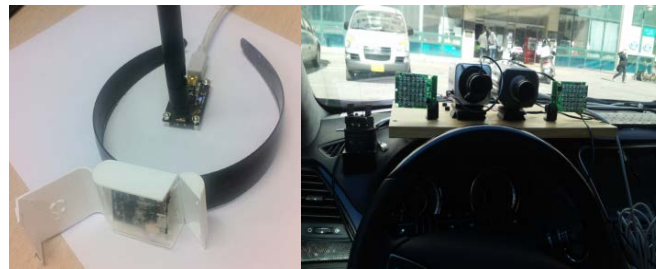
Figure 8. A wireless gyro-sensor module mounted in a white box and its receiver ( left ), and cameras and other setup installed in the vehicle ( right ).
