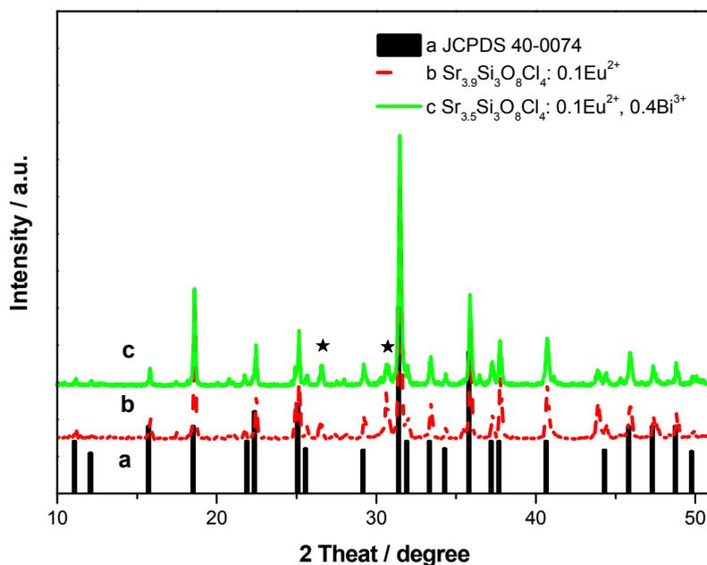
**Figure 1.** X-ray powder diffraction (XRD) patterns of  $\text{Sr}_{3.90}\text{Si}_3\text{O}_8\text{Cl}_4:0.10\text{Eu}^{2+}$  and  $\text{Sr}_{3.50}\text{Si}_3\text{O}_8\text{Cl}_4:0.10\text{Eu}^{2+}, 0.40\text{Bi}^{3+}$ . The Asterisk represents the peak of  $\text{SrSiO}_3$ .
