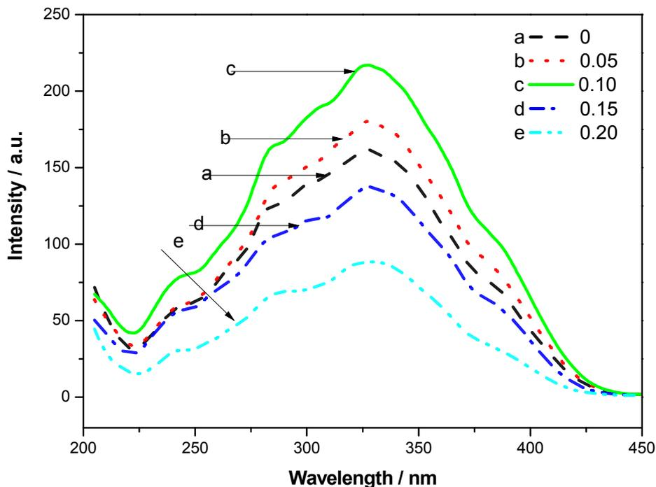
**Figure 4.** Excitation spectra of  $\text{Sr}_{3.90-4y}\text{Si}_3\text{O}_8\text{Cl}_4:0.10\text{Eu}^{2+}, 4y\text{Bi}^{3+}$  ( $y = 0.00, 0.05, 0.10, 0.15, 0.20$ ) by monitoring emission at 490 nm.
