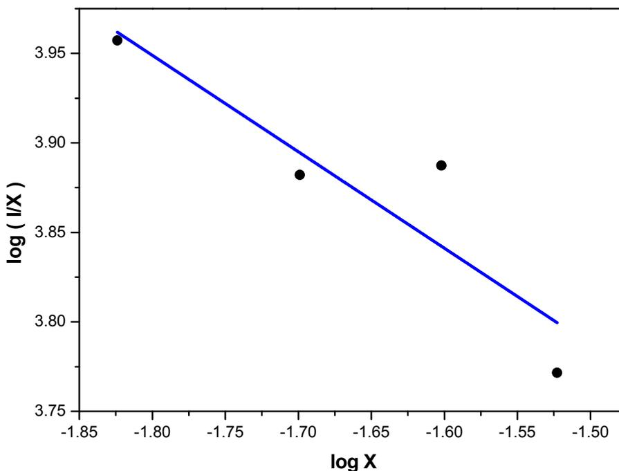
**Figure 3.** The plot of  $\log(I/x)$  as a function of  $\log(x)$  for the  $\text{Sr}_{4-4x}\text{Si}_3\text{O}_8\text{Cl}_4:4x\text{Eu}^{2+}$  phosphors ( $\lambda_{\text{ex}} = 320 \text{ nm}$ ).
