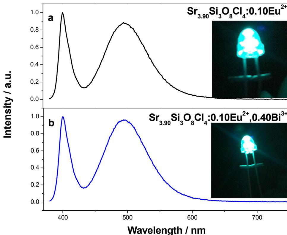
**Figure 6.** Electroluminescence (EL) spectra of the blue-green light-emitting-diodes (LEDs) based on (a)  $\text{Sr}_{3.90}\text{Si}_3\text{O}_8\text{Cl}_4:0.10\text{Eu}^{2+}$  and (b)  $\text{Sr}_{3.50}\text{Si}_3\text{O}_8\text{Cl}_4:0.10\text{Eu}^{2+}, 0.40\text{Bi}^{3+}$  under 20 mA current excitation; the inserted figures are the images of these two LEDs.
