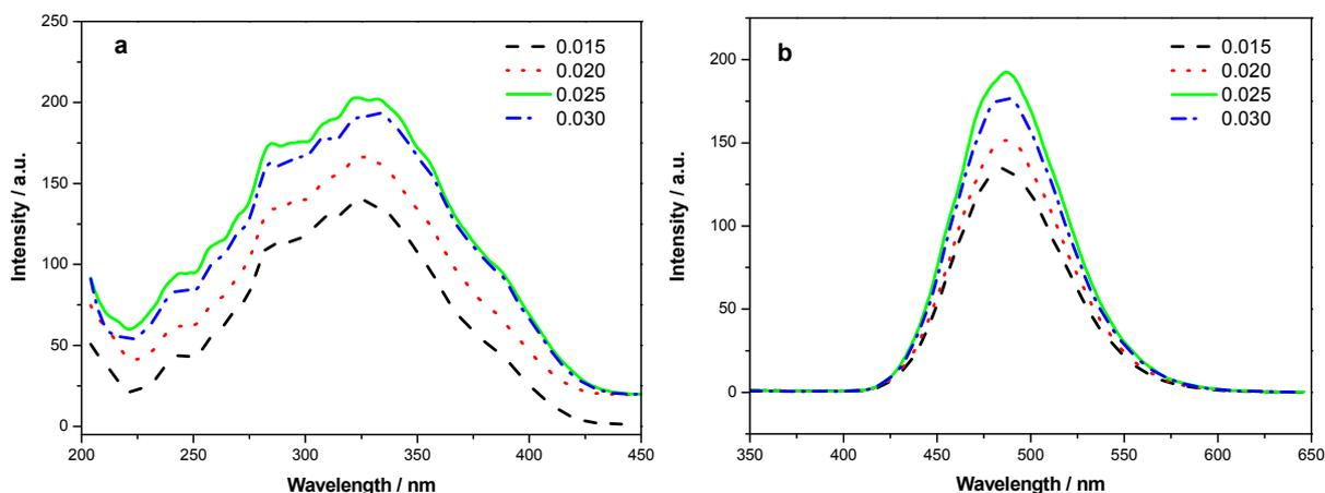
**Figure 2.** (a) Excitation spectra and (b) emission spectra of  $\text{Sr}_{4-4x}\text{Si}_3\text{O}_8\text{Cl}_4:4x\text{Eu}^{2+}$  ( $x = 0.015, 0.020, 0.025, 0.030$ ).
