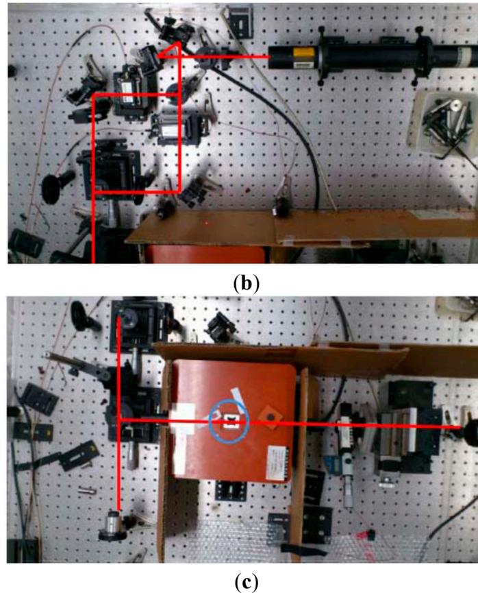
**Figure 1.** (a) Schematic diagram of the optical displacement-enhanced heterodyne polarimeter and sampling system; (b,c) show photos of real experimental apparatus and setup. M: mirror, BS: beamsplitter, PBS: polarizing cube beamsplitter, PhD: photodetector, SBC: Soleil-Babinet compensator, HWP: half-wave plate, AOM: acousto-optic modulator, Pol: polarizer, TEC: thermoelectric cooler, LIA: lock-in-amplifier, PC: personal computer.
