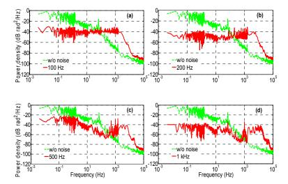
**Figure 3.** Excess phase noise spectra with (solid) and without (dashed) external acoustic perturbations with 80 m polarization maintaining fiber (PMF) being used. Measurement is done at four single-tone perturbation frequencies: (a) 100 Hz; (b) 200 Hz; (c) 500 Hz; and (d) 1 kHz.
