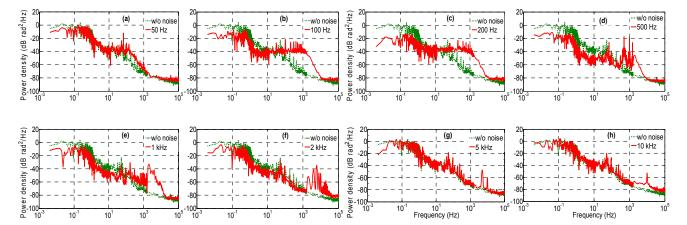
**Figure 2.** Excess phase noise spectra with (solid) and without (dashed) external acoustic perturbations. Measurement is done with 80 m single-mode fiber (SMF) at eight single-tone perturbation frequencies: (a) 50 Hz; (b) 100 Hz; (c) 200 Hz; (d) 500 Hz; (e) 1 kHz; (f) 2 kHz; (g) 5 kHz; and (h) 10 kHz. The driving power is the same for all the frequencies.
