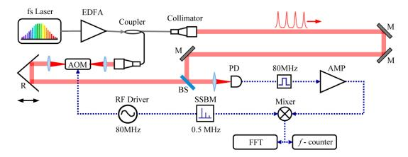
**Figure 4.** Schematic of the outdoor optical frequency transmission test system. AMP: microwave amplifiers, AOM: acousto-optic modulator, BS: beam splitter, EDFA: erbium-doped fiber amplifier, M: silver mirrors, PD: photodetector, R: retro-reflector, and SSBM: single-side band modulator.
